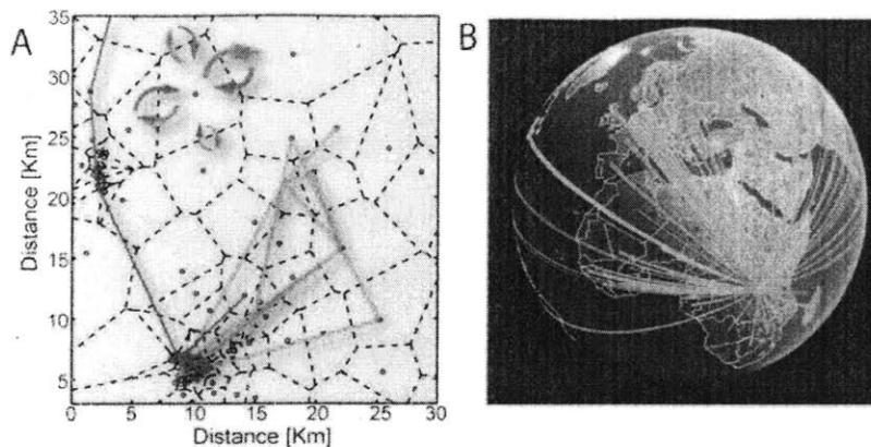
Figure 1-1: (A) Location resolution: Each circle represents a mobile-phone tower and the dashed lines correspond to a Voronoi diagram that roughly delimits the main reception zone of each tower, partitioning the space into individual cells. The blue and red solid lines show the trajectory of two mobile-phone users, illustrating how the call activity helps us to track individual motion. (B) Global analysis: Preliminary results showing the calling pattern between Ruanda and the rest of the world.
