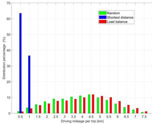
Fig. 10. Driving mileage per charging trip.
