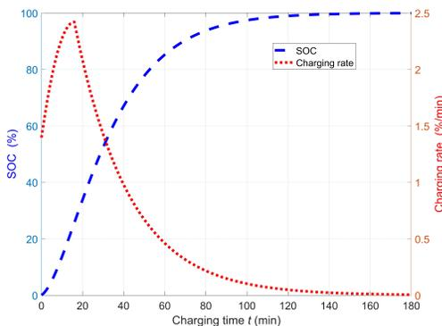
Fig. 3. Charging curve for DC charging method. The parameters setting is from [31]
