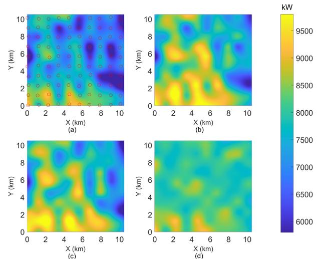
Fig. 5. Heat maps of the power load at 20:00 under different charging station recommendation strategies: (a) initial load (no EV charging), (b) the RMS, (c) the SDMS, and (d) the proposed LBMS.
