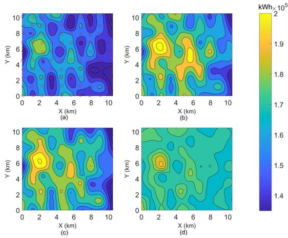
Fig. 6. Contour plots of accumulated daily energy consumption distribution under different charging station recommendation strategies: (a) initial load (no EV charging load), (b) the RMS, (c) the SDMS, and (d) the proposed LBMS.
