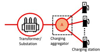
Fig. 2. An illustration of the charging aggregator in a microgrid. All charging stations within the same microgrid are connected to a charging aggregator which can be either a power flow aggregator or a virtual one which is functionally played by the transformer of the substation in the microgrid.
