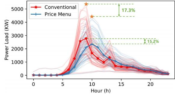
Fig. 13. Charging Load Shifting.
