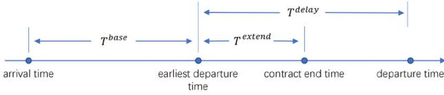
Fig. 2. Illustration of the service process.
