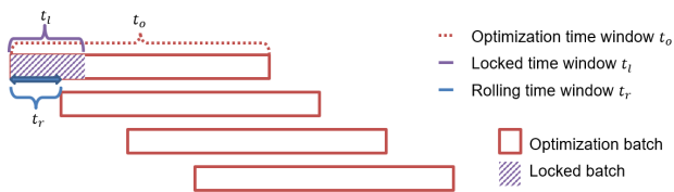
Fig. 2. Illustration of online receding horizon control algorithm structure.
